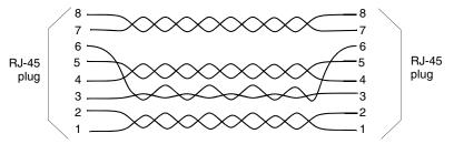
FIG. 12 RJ-45 wiring diagram
